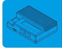
Size Specifications: Height: 29mm Width: 93mm Depth: 71mm Weight: 440G Power Usage <10w
